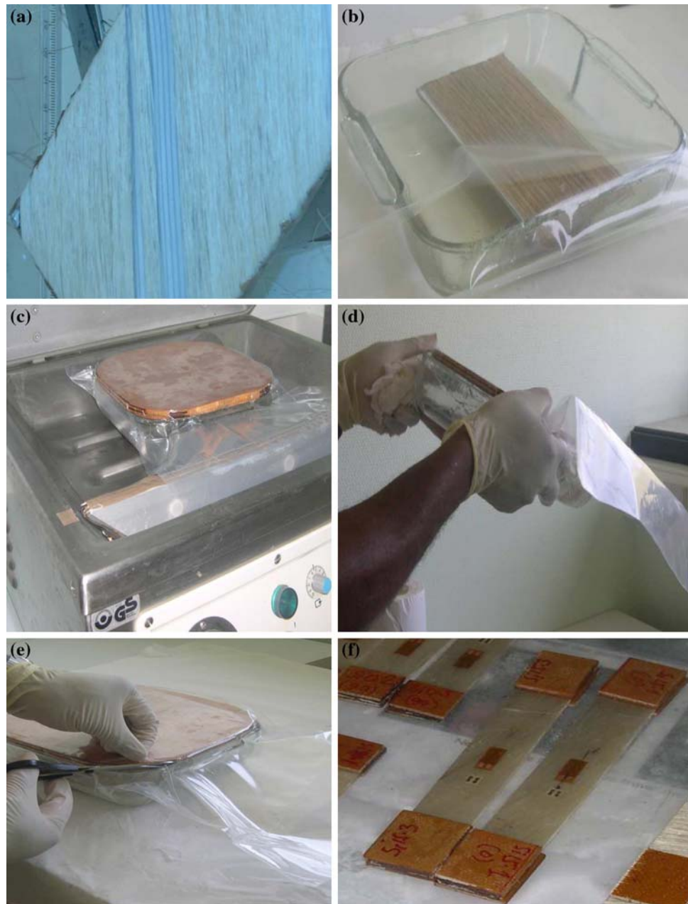
Fig. 3 Composites manufacturing stages. (a) Wrapping of fibres on a glass plate; (b) vacuum setting: stage 1; (c) vacuum setting: stage 2; (d) vacuum setting: stage 3; (e) vacuum setting: stage 4; (f) preparation of UD-composites specimens
